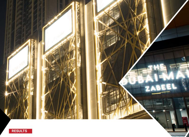
The LED system was powered by 24V Meanwell power supplies, mounted up to 20-30m away. Typically, cable distances of this length are not possible with 24V, as there can be voltage drop, meaning the furthest LEDs do not receive enough volts and there's a drop off in lumen output.
