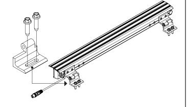
2 Set the angle of fitting and tighten bolts
