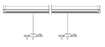
2 Brackets should be spaced equally. The gap between the brackets should be a minimum of 1/3 the length.
