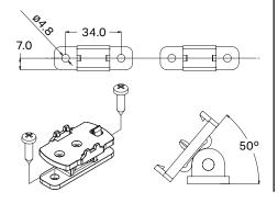
2 Push Azuna fitting into snap fit bracket.
