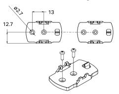
2 Push Azuna fitting into snap fit bracket.
