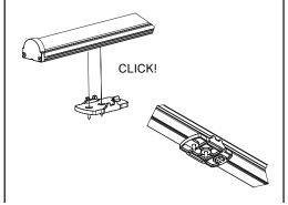
3 if adjustment needed, slide fitting to desired position.
