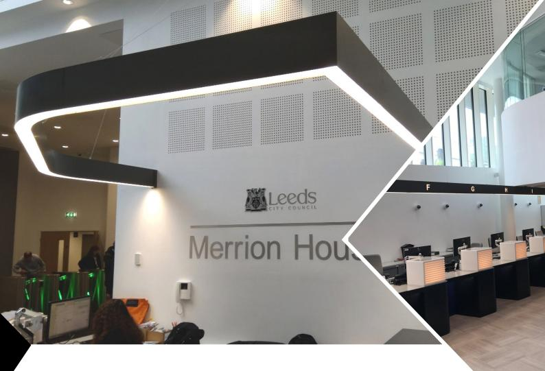
Following successful tests, our engineers produced the full set of 3D drawings. The finished design was CNC laser cut, assembled and installed in modules, which helped the process move quickly and minimised disruption to the site.
