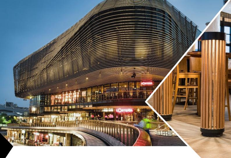
The second fixture was an illuminated bollard made from timber, acrylic and aluminium with an internal LED 3000K cob and heatsink. Again, the concept was designed and presented by GSA, and our team were tasked with creating a more detailed design from which to manufacture the fittings.
