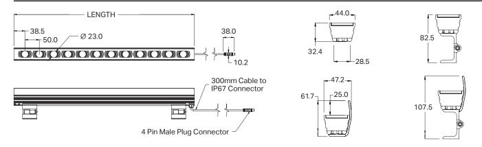
Alphaeus 3 fittings are provided with a 300mm cable with male plug connector. Extension cables with female socket connector must be purchased separately with the below product codes.
