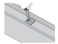
Incrementally pull each suspension cable through its respective clutch until the fitting reaches the desired height.
