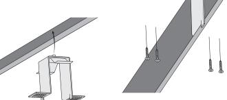
If there are multiple profiles, insert the top joining plate and 2x side joining plates halfway into the profile end. Connect the mating profile and tighten the 4x grub screws in the top plate to lock the profiles together.
