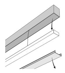
Using the included M5 bolts, fasten the profile to the brackets. Incrementally tighten all bolts until the profile engages the bracket springs. Continue tightening until the bottom edges are at finished ceiling level.
