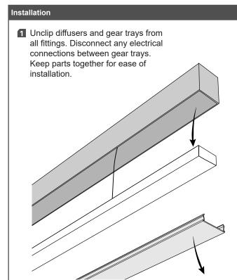
Clip all gear trays back into the profiles as indicated whilst reconnecting any electrical connections. Take care not to trap any cables when inserting gear trays. Complete all earth connections by inserting the profile earth cable into the Wago connectors on the corresponding gear tray.
