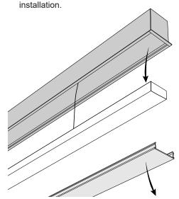
4 Tighten bolts inside the fitting extrusion profile until the bracket twists into locked position. Continue tightening until flange is tight against ceiling.
