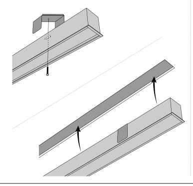
2 Unclip diffusers and gear trays from all fittings. Disconnect any electrical connections between gear trays. Keep parts together for ease of
