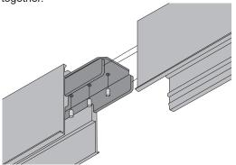
Clip all gear trays back into the profiles as indicated whilst reconnecting any electrical connections. Take care not to trap any cables when inserting gear trays. Complete all earth connections by inserting the profile earth cable into the Wago connectors on the corresponding gear tray.
