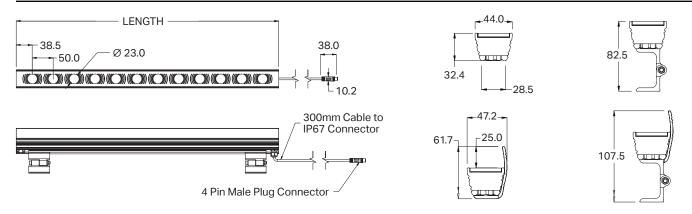
Alphaeus 3 fittings are provided with a 300mm cable with male plug connector. Extension cables with female socket connector must be purchased separately with the below product codes.
